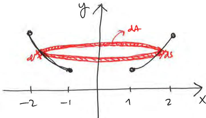
$$\begin{aligned} dA &= 2\pi \times ds \\ &= 2\pi \left( x^2 + \frac{1}{4} \right) dx \end{aligned}$$
