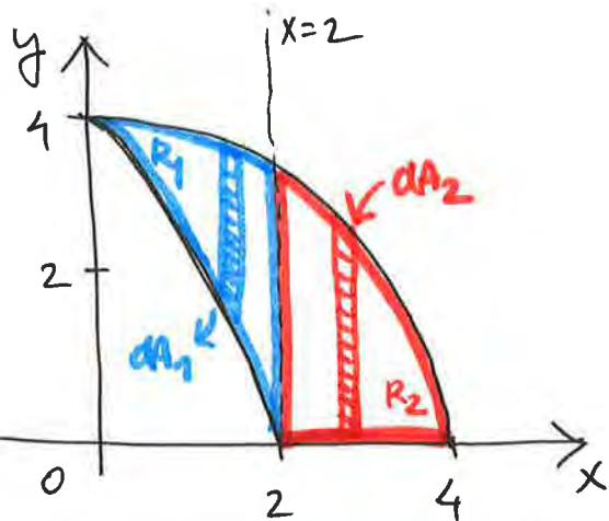
$$\begin{aligned} dA_1 &= (y_{c_1} - y_{c_2}) dx \\ &= (\sqrt{16-x^2} - 4+x^2) dx \end{aligned}$$
